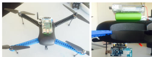
Figure 2. The repairing agent: the Iris+ drone carries the Pi on top and the EPM (with a sensor node) at bottom.
