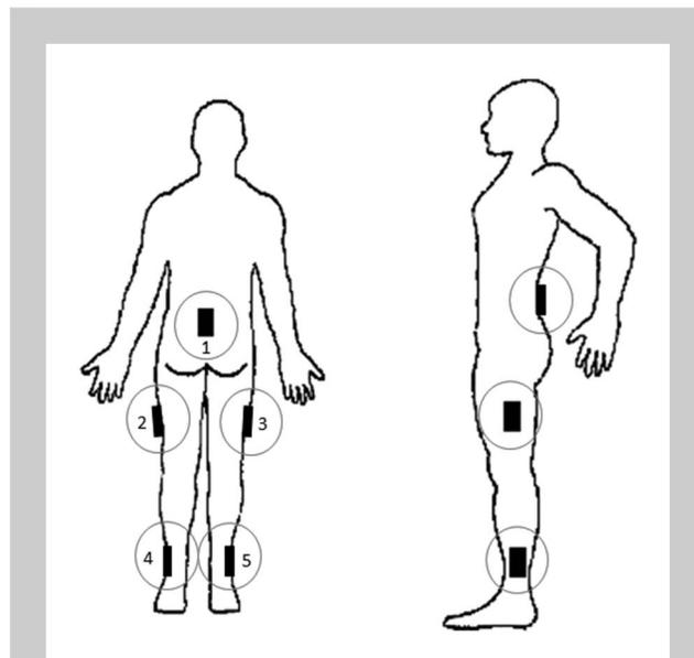
**Figure 1.** The 5 IMU positions: (1) spinous process of the fifth lumbar vertebra, (2 and 3) mid-point of both femurs on the lateral surface (determined as halfway between the greater trochanter and lateral femoral condyle), (4 and 5) and on both shanks 2 cm above the lateral malleolus.
