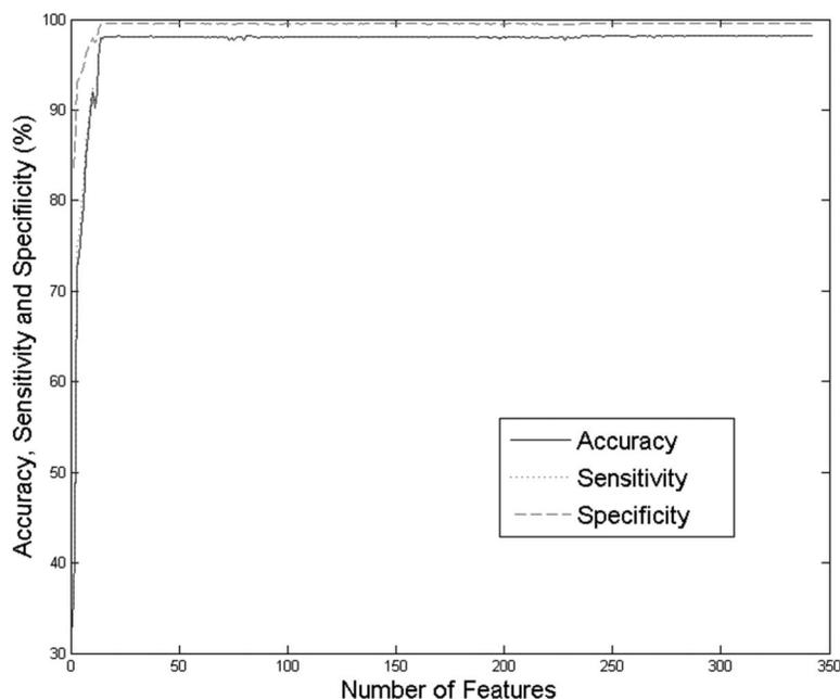
**Figure 7.** Graph showing accuracy, sensitivity, and specificity of exercise classification with the right shank IMU using 1–324 of the available features, ranked in the order of importance.
