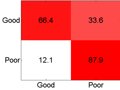
Figure 2: Heatmap confusion matrix showing binary classification results with right thigh sensor. Rows show the actual class of a repetition and columns show the classifier’s prediction
